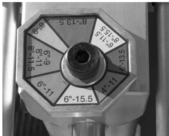
This stop position (at bottom) is set to squeeze 6" 15.5 DR pipe. Stops on both sides of tool must match for proper use. And, desired setting must be in this bottom orientation.
